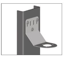
**1b.** Mounting Method 2: Secure wall mount bracket to mounting surface using customer supplied screws, flat washers, and nuts.
