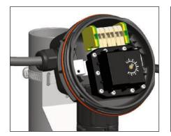
Install complete system wiring. Terminal set screws shall be tightened to a torque value of 1.4 Nm (12.4 lb-in). See Step 4 for wiring details. Set thermostat at desired set point (Winterization=5°C).
