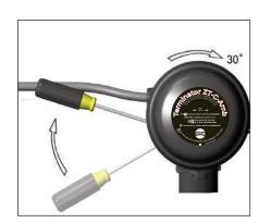
6. Use screwdriver to ratchet on junction box lid. Lid will rotate 30 degrees. To remove lid, repeat steps 14 and 15 but in the opposite direction.
