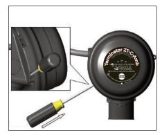
5. Install junction box lid and twist hand tight. Insert screwdriver into ratchet slots located on side of junction box base.
