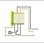
**4.** Wiring Details: Thermostat Connection.
