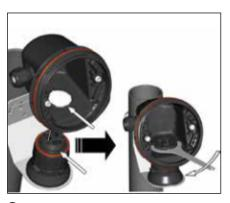
**3.** Mount junction box base on expediter. Make sure to align slots to properly orient junction box base. Tighten nut with Terminator-LN-Tool.
