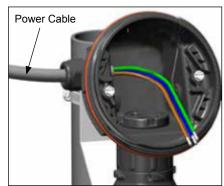
**5.** Install power cable and RTD. Stainless steel RTD tip must extend ≥ 20 mm out of gland.
