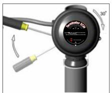
**8.** Use screwdriver to ratchet on junction box lid. Lid will rotate 30 degrees. To remove lid, repeat steps 7 and 8 but in the opposite direction.
