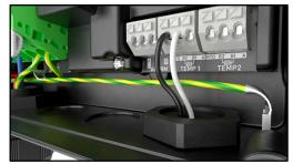
f. Tighten the cable gland cap by rotating clockwise applying the recommended torque.
