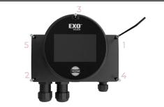
c. Remove the cover carefully. The board-to-board cable is connected by a zip tie at each end. Avoid straining the wire between the base and the cover.
