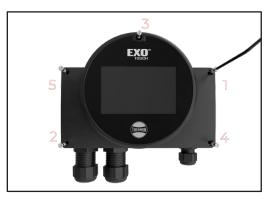
c. Tighten the captive screws using 9-in-lbs torque.
