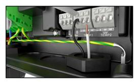
Note: When using a single thermistor, connect to terminal labelled TEMP1.
