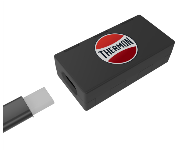
14. Push the end seal onto the heat trace cable until the overjacket is fully contained within the end seal.
