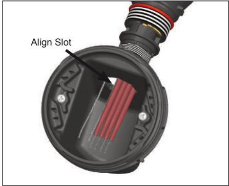
18. Mount junction box on expediter making sure to align slots to properly orient junction box base.
