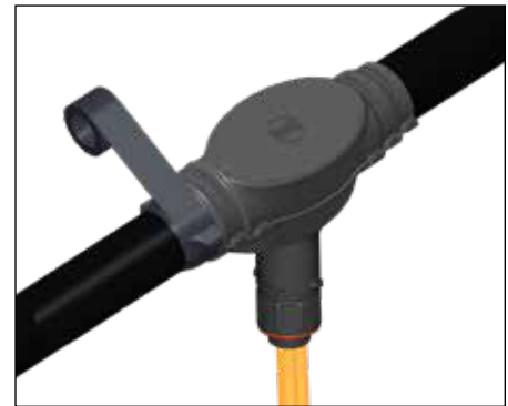
15. Apply self-vulcanizing tape around bundle jacket and work up over FAK ends.
