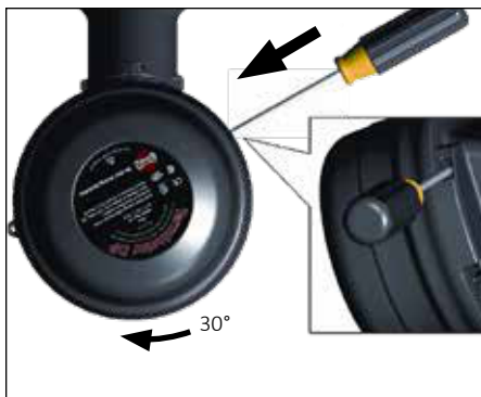
20. Install junction box lid and twist hand tight. Insert screwdriver into ratchet slot located on side of junction box base to tighten. Use screwdriver ratchet on junction box lid. Lid will rotate 30°.
