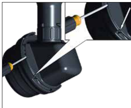
21. Lid latch mechanism fully engaged. To remove lid, repeat step 20 but in opposite direction.
