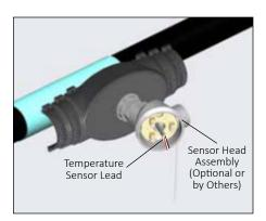
7. If applicable, connect sensor head assembly to the sensor cover bottom using the supplied hardware. Be sure temperature sensor lead is guided through the opening found in the middle of the terminal mount.
