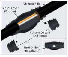
4. Using the dimensions on the sensor covers, locate the correct size, ensuring a snug fit. Identify the correct cut lines, and cut top and bottom sensor cover ends.
