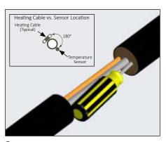
Prepare tubing bundle for temperature sensor by inserting a phillips screwdriver between the process tube(s) and insulation at a point opposite the heating cable. The sensor should be placed 180° around the circumference from the heating cable. Make sure that the entire length of the sensor is in intimate contact with the tube surface. Prevent kinking.
