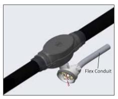
**11.** If applicable, connect flex conduit to sensor head assembly using hardware supplied by others. Be sure to guide power wires through opening found in the middle of the terminal mount.
