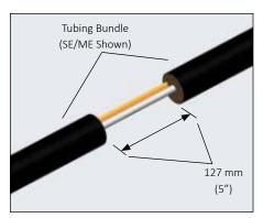
1. Remove outer jacket and insulation from tubing bundle approximately 127 mm (5") to expose the process tubes and heat trace.
