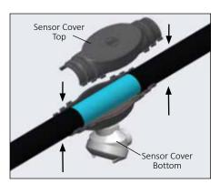
**9.** Assemble sensor top, tubing bundle, and sensor bottom together as shown. Snap both halves together firmly. Inspect cover ends for snug fit. Apply additional RTV sealant where needed.
