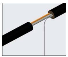
**3.** Insert the temperature sensor into the prepared hole in the thermal insulation. Ensure contact is maintained with the tube.
