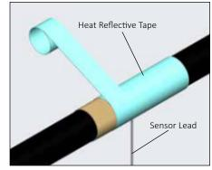
**6.** Complete with additional passes of heat reflective tape.
