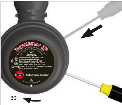
17. Install junction box lid and twist hand tight. Insert screwdriver into ratchet slot located on side of junction box base to tighten. Lid will rotate 30°.
