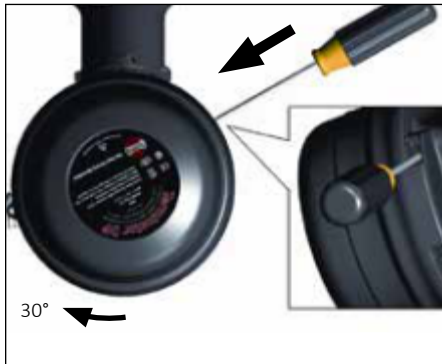
16. Install junction box lid and twist hand tight. Insert screwdriver into ratchet slot located on side of junction box base to tighten. Use screwdriver ratchet on junction box lid. Lid will rotate 30°.
