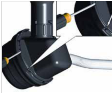
17. Lid latch mechanism fully engaged. To remove lid, repeat step 15 but in opposite direction.
