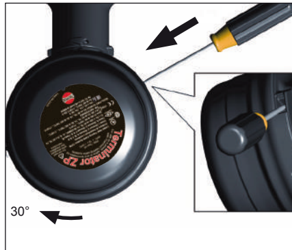
19. Install junction box lid and twist hand tight. Insert screwdriver into ratchet slot located on side of junction box base to tighten. Use screwdriver ratchet on junction box lid. Lid will rotate 30°.
