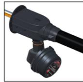
**Terminator DP/FAK-1 Kit** for bulkhead entry of electrically heated TubeTrace bundles. The kit is designed to make a waterproof seal over the end of TubeTrace and terminate Thermon electric heat tracing in an approved junction box. Kit will make one connection. (PETK termination kit for electric heat tracing required, order separately).
