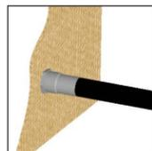
Bulkhead Entry Heat Shrink Seal provides an effective transition and strain-relief when bundle passes through a wall 1" thick or less.
