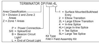
DP/FAK and ZP/FAK Power Connection/Splice Kits are designed to fabricate power connections, in-line/T-splice connections or for making end terminations on TubeTrace with electric heat tracing. (PETK/SCTK termination kit required, order separately)
