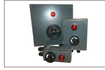
**CS-L\*-Ex....** Circuit switch with lamp to be used as an in-line isolation switch for single phase, phasephase and 3-phase heat tracing circuits. Available in 16 A, 25 A and 40 A versions.
