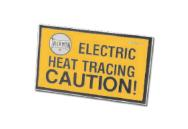
**CL**...vinyl-based peel-and-stick caution labels are intended for direct exposure to industrial environments. Electrically heated pipelines and vessels should be clearly identified at frequent intervals along the pipeline or vessel. Caution labels should be placed at 3 to 6-m intervals or as required by code or specification. Additional languages or other texts are available; contact TC-E.
