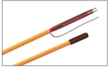
**PETK...**circuit fabrication kits are required for use with all Thermon Parallel Heating Cables Connection Kits. Kits for termination of SX cables include a power connection boot, end cap, RTV adhesive and a caution label. Kits for termination of HPT and FP cables also include tape strip and a distinct grommet.
