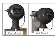
**Terminator ZP**... is designed to fabricate power connections, in-line/T-splice connections or for making end terminations. The Terminator ZP-XP is suitable for use in hazardous areas (Ex e T6/T4), harsh industrial environments and has a IP66 rating. The up front positioning of the terminal block permits easy access during termination and for future routine maintenance.
