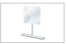
**XP-1-...**predrilled stainless steel (type 304) mounting bracket designed for mounting Thermon junction boxes and thermostats directly to the pipework. The bracket is easily secured to the pipe using B-4, B-10 or B-21 attachment bands. The XP-1 utilizes a 110-mm standoff.
