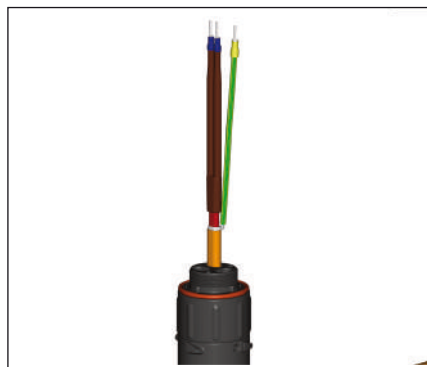
7. Terminate cable with appropriate PETK termination kit. Refer to PETK installation instructions.
