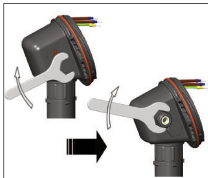
10. Install M25 power gland (order separately) and M25 blind plug. For in-line splice, T-splice, or end termination, install additional M25 blind plug (order M25-B-EXE separately) instead of M25 power gland.
