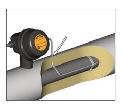
**16.** Seal temperature sensor penetration through insulation cladding. For ambient sensing applications, the mounting location should be representative of the coldest region, and the sensing element should not be exposed to direct sunlight or any additional heat source.
