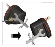
7. Install M20 blind plugs in remaining M20 threaded entries.
