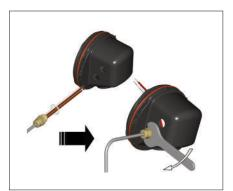
**5.** Place M20 sealing washer on temperature sensor gland connector. Route temperature sensor leads through M20 threaded entry. Screw gland connector into junction box.
