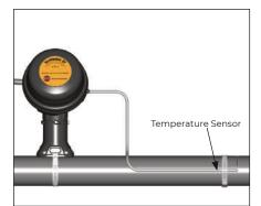
**15.** Mount the temperature sensor securely to the pipe using pipe band. Make sure the entire length of the sensor is in intimate contact with the pipe. The sensor should be placed at least 90° around the circumference from the heating cable.
