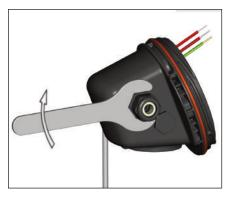
**8.** Install M25 power gland in M25 threaded entry. (Customer Supplied)
