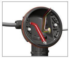
Install control wiring (user supplied, 6 mm² max). 3 wire cable (for 1 sensor) or 6 wire cable (for 2 sensors) with braided earth shield is recommended.
