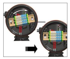
**10.** Install quick mount terminal blocks and tighten screws (if necessary).
