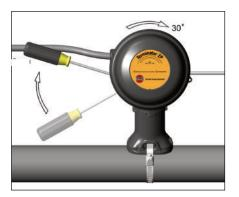
13. Use screwdriver to ratchet on junction box lid. Lid will rotate 30 degrees.
