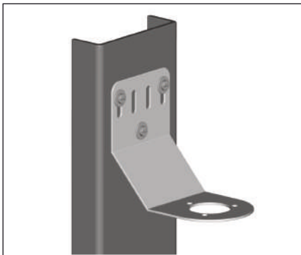
1b. Mounting Method 2: Secure wall mount bracket to mounting surface using screws, washers, and nuts (customer provided)
