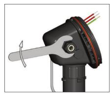
Install M25 power gland (customer supplied) in M25 threaded entry. For in-line splice or 3 phase wye connection, install M25 blind plug (order M25-B-EXE separately) instead of M25 power gland.
