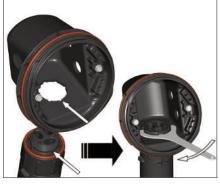
4. Mount junction box base on expediter. Make sure to align slots to properly orient junction box base. Tighten nut with Terminator-LN-Tool. If mounting horizontally, threaded gland holes must face downward.
