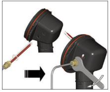
Route MI cable cold leads through M20 threaded entries. Screw cable glands into junction box.
