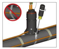
10. Mount expediter to pipe using pipe band. Do not band over cable. If necessary, temporarily mount junction box base on expediter.
