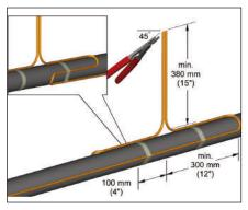
1. Cut end of cable at angle to aid in piercing grommet. Leave additional cable for expansion loop.
