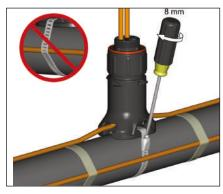
Temporarily mount expediter to pipe using pipe band. Do not band over cable.
