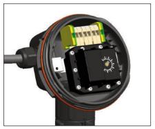
16. Install thermostat and complete system wiring. Terminal set screws shall be tightened to a torque value of 1.4 Nm (12.4 lb-in). See page 4 for wiring details. Set thermostat at desired setpoint.
