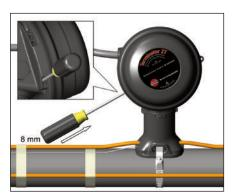
17. Install junction box lid and twist hand tight. Insert screwdriver into ratchet slots located on side of junction box base.
