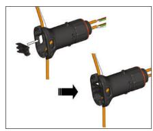
**9.** Insert banding guide and snap into place.
