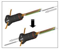
8. Route thermostat bulb through nut and expediter opening in junction box base. If necessary, apply lubricant (user supplied) to end of thermostat bulb. Slide through conical grommet hole. Push excess capillary tube through expediter.
