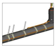
**12.** Fix thermostat bulb and capillary tube to pipe.
