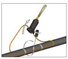
**7.** Remove expediter from pipe by removing pipe band.
