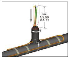
11. Push excess cable and capillary tube back through expediter. Tighten cap securely. Tape cable expansion loop to pipe.
