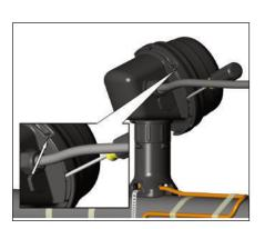
**19.** Lid latch mechanism fully engaged. To remove lid, repeat steps 17 and 18 but in the opposite direction.
