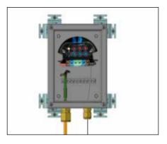
**6.** Terminate cable with appropriate PETK termination kit. Refer to PETK installation instructions. Push excess cable back through gland. Tighten cap securely. Tape cable expansion loop to pipe.
