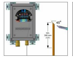
**4.** Locate bus connection (HPT and FP only) as shown. Cut end of cable at angle to aid in piercing grommet. Leave additional cable for expansion as needed.
