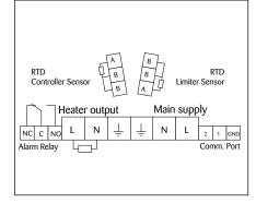
**9.** Wiring Details: Connect ground wire from power cable, braid from heater, and connections from the module to the grounding strip.
