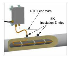
**13.** Install IEK insulation entry kit to seal heating cable and RTD lead wire penetrations through insulation cladding.
