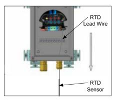
**3.** Position RTD Sensor(s) in grommet. Do not pull from the sensor end when routing through the RTD gland. Pull sensor from the lead wire portion.
