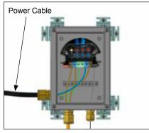
8. Install power cable. Complete system wiring. Terminal set screws shall be tightened to a torque value of 1,4 Nm (12,4 lb-in). See wiring details. Set modules electronic control and/or control limiter at desired setpoints.
