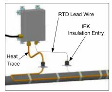
**12.** Slide IEK insulation entry kit onto RTD lead wire. Fix RTD lead wire and sensor to pipe.
