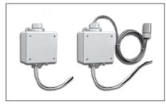
**STC-DS-2B**...stand-alone snow and ice sensor/controller is designed to operate on either 120 Vac or 208-240 Vac control power, includes a single 30 A normally open load contact rated to 277 Vac, and provides an adjustable temperature set point with manual on/off, automatic and standby switching functions.
