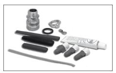
**RGS-CFK...**circuit fabrication kit is designed to fabricate an RGS circuit with one power connection boot and one double end cap. The kit includes a cable transition fitting with watertight grommet and RTV adhesive. Power connection must be made in a NEMA 4, UL Listed junction box (not included).
