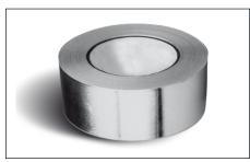
**AL-20L...**aluminum tape for securing cable in the bottom of a gutter. Tape is designed to hold cable in place and prevent movement during heavy rains. Allow one foot of tape for each foot of heating cable. Tape is 2" (51 mm) wide x 150' (46 m) long.
