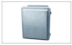
KSR-JB...nonmetallic junction box is intended for use with KSR cables. Heating cables enter the junction box through rigid conduit (not included) from the area to be heated. Constructed of corrosion-resistant materials, the NEMA 4X unit includes a hinged and lockable cover.
