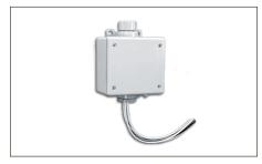
STC-DS-2B...stand-alone snow and ice sensor/controller is designed to operate on either 120 Vac or 208/240 Vac control power, includes a single 20 Amp normally open load contact rated to 277V, and provides an adjustable temperature set point with manual on/off, automatic and standby switching functions.
