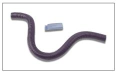
KSR-EJK...expansion joint kit is designed to allow cable to cross a concrete expansion or construction joint. When installed, the kit will allow normal expansion and contraction of the substrate without straining or damaging the heating circuit. Easy-to-use kit includes a reinforced flexible sleeve and RTV adhesive.
