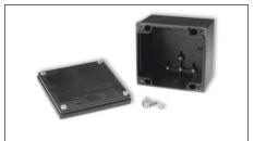
**JB-K** nonmetallic junction box is intended for use with the PCA-COM kit. The corrosion-resistant NEMA 4X unit includes a removable gasketed cover and ground lug.
