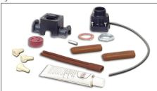
**PCA-COM** circuit fabrication kit is designed to fabricate an HSX 2100 circuit with one power connection boot and one end cap. Up to three HSX heat tracers can enter a junction box supported by a PCA-COM kit when additional connection boots (TBX-3L) and end caps (ET-6) are used.
