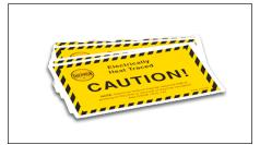
**CL** caution labels (vinyl-based peel and stick) should be installed on the thermal insulation weather barrier. In accordance with the NEC, electrically heated pipelines and vessels are to be clearly identified "at frequent intervals along the pipeline or vessel." Caution labels should be placed at 3-6 m (10'-20') intervals or as required by code or specification.
