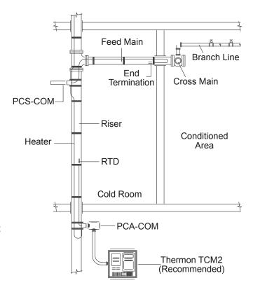
In case of dry type, the tracing is meant to keep the empty branch pipes above freezing point, so that when upstream control valve operates the pipe body does not cool down the incoming water.
