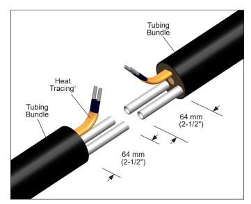
1. Strip back insulation approximately 2.5 in. (64 mm) from the end of the Pre-insulated Tube Bundle.
