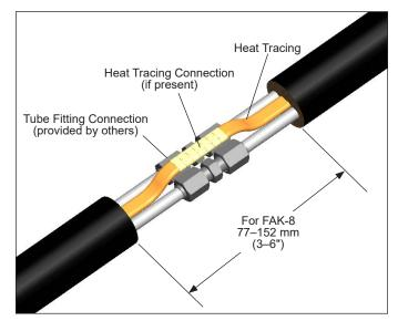
Make connections with appropriate fittings 2. (provided by others). Test fittings for leaks before proceeding. If tubing bundle includes heat trace, make splice per kit instructions included with heat tracing.
