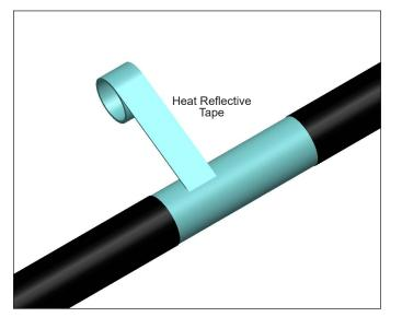
3. Wrap tube(s) with 1 pass of heat reflective tape (25% overlap). Then wrap with 3 passes of glass fiber tape (50% overlap). Complete with 1 additional pass of heat reflective tape.
