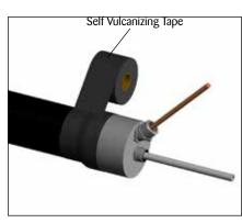
**6.** Wrap the self vulcanizing tape around the bundle jacket. Continue wrapping the tape around the bundle and end cap making sure to overlap each wrap by 50%.
