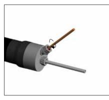
**11.** Tighten fitting nut to compress grommet against the heat tracer(s).
