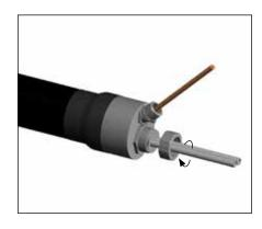
**15.** Slide the tube fitting nut over the tubes and tighten, compressing the packing material and washers together.
