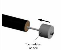
**20.** Remove fitting nut. Slide the ThermoTube end seal over the tube.
