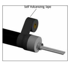
**28.** Wrap the self vulcanizing tape around the bundle jacket. Continue wrapping the tape around the bundle and end cap making sure to overlap each wrap by 50%.
