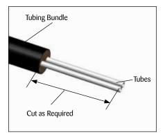
**24.** Remove outer jacket and insulation from the end of the tubing bundle.
