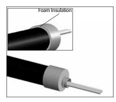
**27.** Slide foam insulation into the area between the tubing bundle end seal and the tubing bundle jacket routing the tubes through their designated openings. Be sure the tubing bundle end seal lid touches the end of the bundle.
