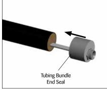
**25.** Remove fitting nuts and grommets. Slide the tubing bundle end seal over the tubing.
