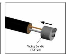
**3.** Remove fitting nuts and grommets. Slide the tubing bundle end seal over the tubing and heat trace. If bundle does not include heat trace, seal should only include a single fitting. Disregard any instructions toward heat trace if not applicable.
