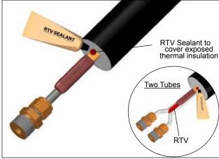
**3.** Liberally apply RTV sealant to tubing bundle insulation. For multi-tubes, apply RTV between the tubes.
