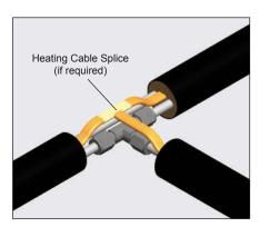
If bundle includes electric heat trace, make-up splice per instruction included with heater cable kit. This should be accomplished after fittings are leak tested.
