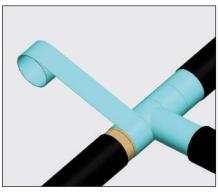
Complete with additional passes of heat reflective tape.
