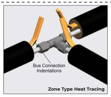
**2a.** If bus connection indentation is less than 38 mm (1.5") from end of the heat tracing, proceed stripping the bundle insulation to the next indentation.
