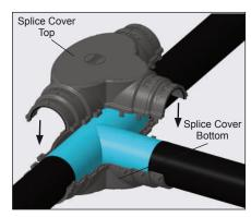
**8.** Fit tubing bundle to bottom half of cover and install top half. Snap together firmly. Inspect ends of tubing splice cover for snug fit. Apply additional RTV sealant where needed.
