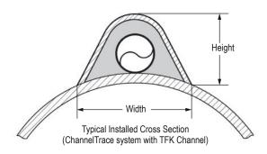
1. Galvanized TFK channels are only used up to 210°C (410°F). Stainless steel channels are required for higher temperatures.
